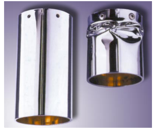
Figure 6: Comparison of exhaust tail pipes (new / after crash)
