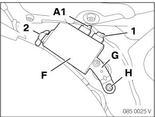
Connect the plug (1) of the converter wiring harness and branch **A1** of the PDC wiring harness into the same coloured plug casing on the PDC control unit **F**.
