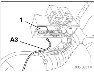
Plug branch **A3** into the free slot in the joint connector **X10116** (1) with colour WSRTGE.
