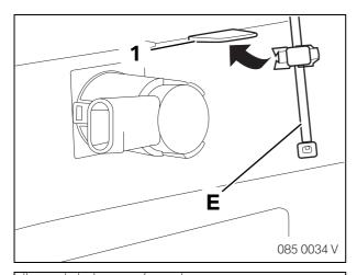
Push cable ties and holders **E** onto the plastic projections (1).
