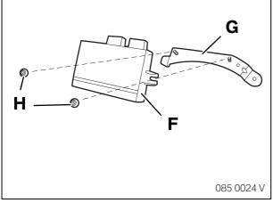
Use plastic nuts  ${\bf H}$  to fit the PDC control unit  ${\bf F}$  onto the holder  ${\bf G}$ .
