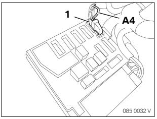
Connect branch **A4** to PIN 13 of plug **X11007** (1) on the power distributor.
