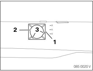
Mark the midpoint within the marks (1) and centrepunch it. Drill holes (2) (Ø27 mm).
