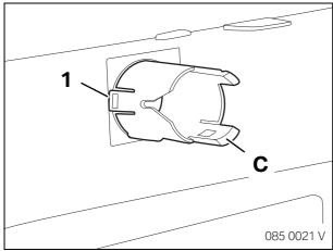
Insert the ultrasonic converter holders **C** into the holes.
