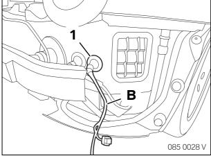
Insert the grommet (1) for the converter wiring harness **B** into the body recess.
