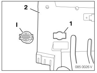
In cars not fitted with a gong I, cut out the recess (1) along the embossed mark on the inside of the pedal trim (2). ◀
